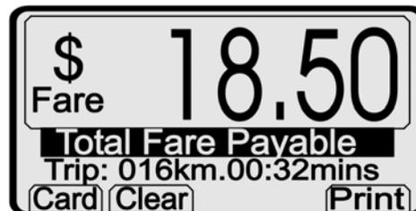
If the meter is equipped with a "Swipe Reader" then it is armed in this mode, ready for a payment card to be swiped. The Banner; "Total Fare Payable" alternates with "Swipe Reader Enabled". When a payment card is swiped, the card type is automatically detected and the appropriate "Service Fee", "Subsidy" or "Discount" applied and displayed on-screen, as shown. ie the screen changes to that shown here. The "Fare to Pay" is calculated by adding the Service fee or subtracting the Subsidy.
