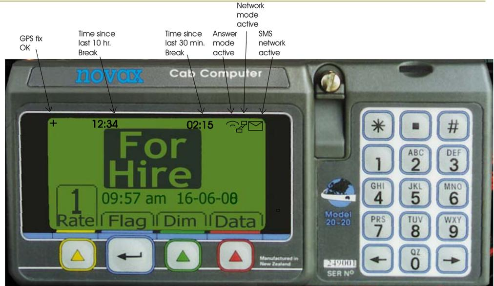
when the appropriate breaks have been taken, ie the meter switched to the "off" mode for the required period (30 minutes/ten hours). "Hours worked" timers accumulate whenever the meter is "For Hire" and "Hired". The third timer logs the time since a 24 hour break was taken, and will only be displayed if this period exceeds 70 hours, in which case the timer will be displayed in place of the other two timers.
