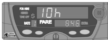
Meter "For Hire", showing working-hours limit has been exceeded, and is thus displayed.
